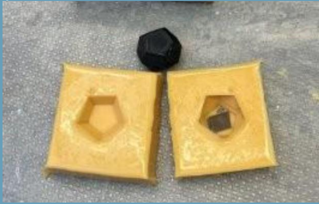
Stage 1 – Initial 3D-printing and silicone mould-making practice using geometric shapes.
