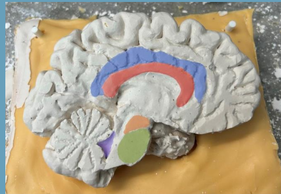
Stage 6 – Final mould was made using a 90% scale resin printed hemisphere model.
